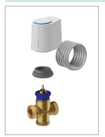
In order to install the actuators **art.1911-1912-1921** on piston valves, remove the manual handle from the valve and screw the appropriate adapter included in the package. Then place the actuator over the adapter and press down until it engages.
