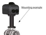
Adapter for actuators installation (ART. 3039-3040) on 1/2"-3/4"-1"-1"1/4 zone valves.
