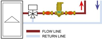
**⚠ For cooling systems the deaerator should be installed in the return line.**
